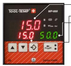
Set temperature / required temperature Adjustable in 1/10° range
